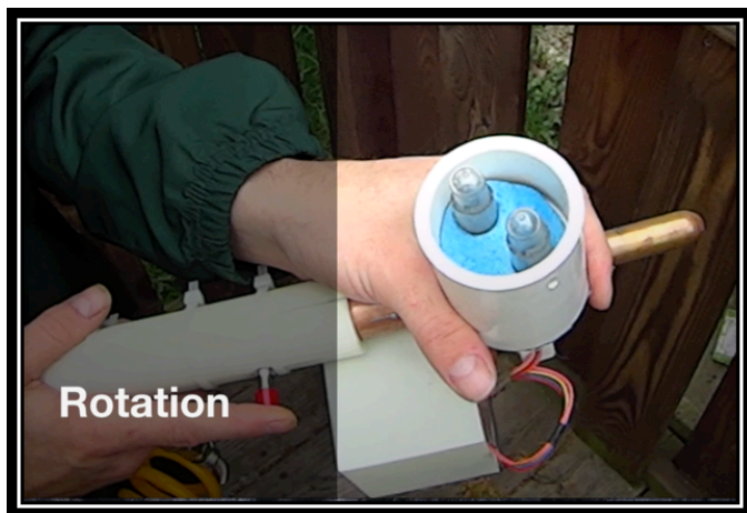
Figure 5: In the figure above, the rotation of the cartridges is initiated when the red button is pressed which activates the stepper motor below the solution holder. The motor rotates the cartridges 90 degrees clockwise.
