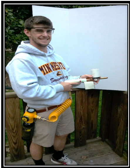
Figure 7: The above image shows the user holding the SprAid device. The CO2 tank is buckled the belt. The user can operate the device by holding on to the elbow joint handle and pushing back on the pipe with the other hand. The device is battery powered and can be operated indoors or outdoors.
